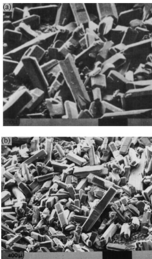
Fig. 6. SEM photographs of the K 2 SO 4 crystals produced by the ammoniation process.
